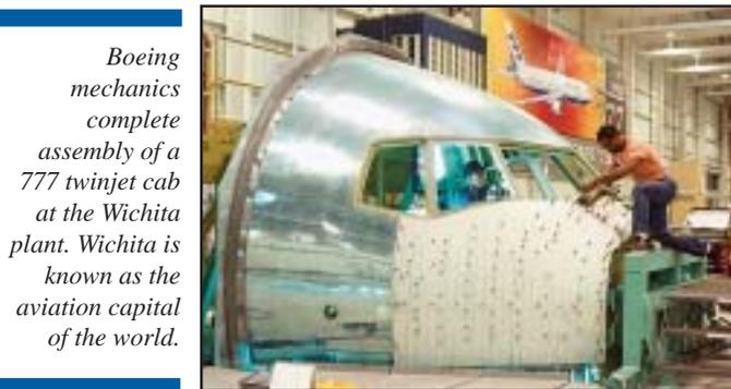
Boeing mechanics complete assembly of a 777 twinjet cab at the Wichita plant. Wichita is known as the aviation capital of the world.
